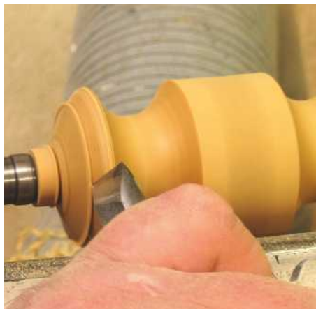
▲ Pic.26 The other end is done with the skew to show that this job could be done with either tool. A slicing cut with the long point of the skew is the safest way, and leaves a superb finish
